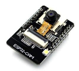
This development board is an ESP32 based board with WiFi and Bluetooth and has a built-in camera. In addition, the board also has a micro SD card connection.
